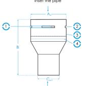
Slide the HT duct flange onto the adapter
