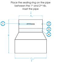
Insert the fitting with sealing ring
